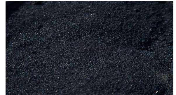
Recycled plastic and crumbed rubber in road surface
